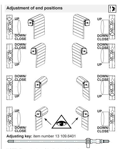
**NOTE:** For activation of the limit switch setting screws, use the setting tool or Phillips/hexagon socket tool. Never use an electric screwdriver!
