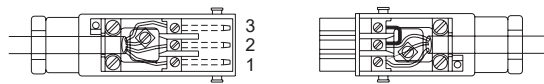
Fig. 5 Circuit diagram RolTop-868 230 V / 50 Hz and wiring at use with Hirschmann plug STAS 3 (with jumper)
