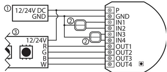
**Note.** The device works in RGBW mode by default, to enable HSB mode change parameter 150 to 1.
