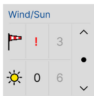
View cable break / loss of sensor
