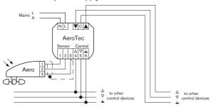
**Note!** Always use a shielded control wire ... o.8 mm or telephone line JY-ST ... o.6 mm.
